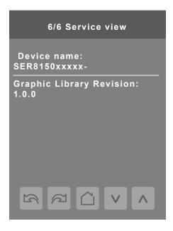
The Model number is the BACnet® device name automatically assigned from factory and is automatically combined with live BACnet instance number. This name can be modified from the BACnet dev Object.
