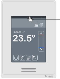
Touch and hold this point for 3 seconds to enter setup mode
